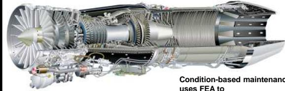
Condition-based maintenance uses FEA to predict component life for components in jet turbine engines such as the F414 powerplant for the F-18E/F Superhornet aircraft.
