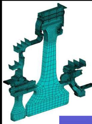
Complex model of the F414 aircraft engine high-pressure turbine rotor was created through ANSYS pre-processing capabilities.
