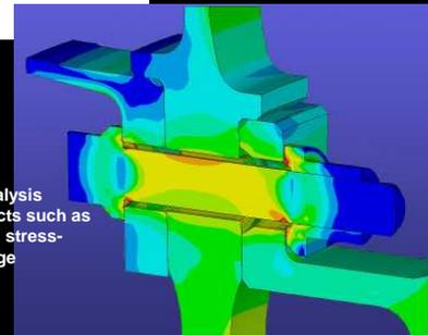
Detailed rotor analysis accounts for effects such as frictional contact, stress-stiffening and large deformations.
